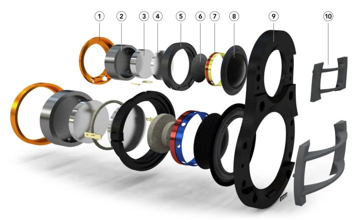
1 CNC-machined aluminium alloy finishing ring.
